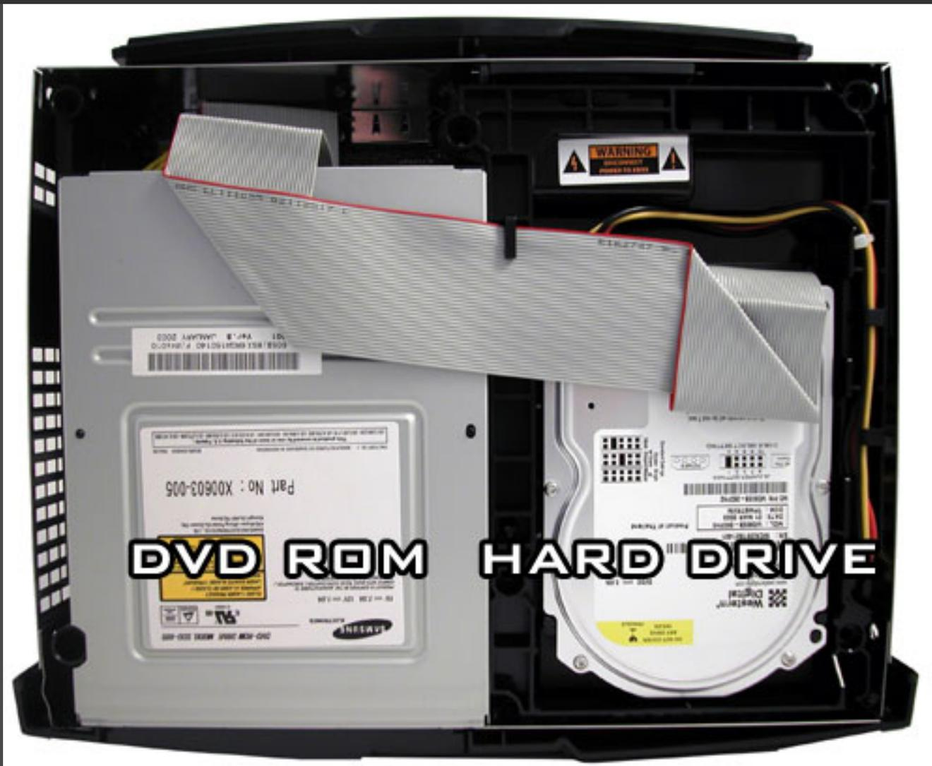
Use the Torx 10 Screwdriver. Unscrew the 3 screws and remove the DVD ROM & Hard Drive units. Unplug the grey IDE cable and yellow power cable from the mainboard.
