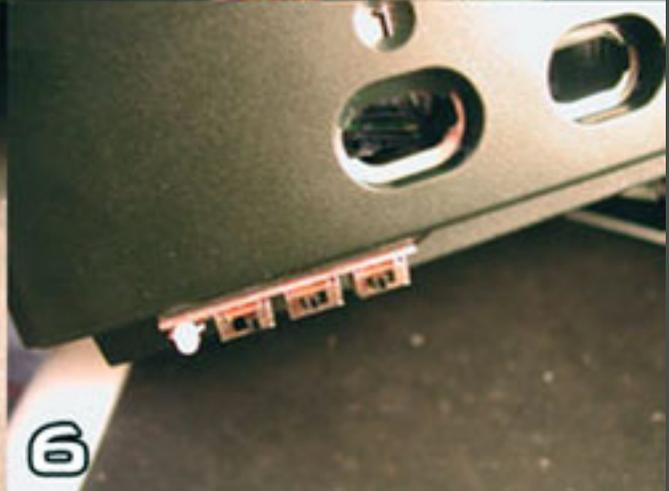
If you are satisfied that everything is connected correctly, set the external switches to Enabled, Unprotected & Bank 1. Plug in the AV and power cables and turn the Xbox on. The LED on the external switch should be green and the 2 blue LED's should light up on the modchip. The power/eject button on the Xbox should flash Green and Orange.
